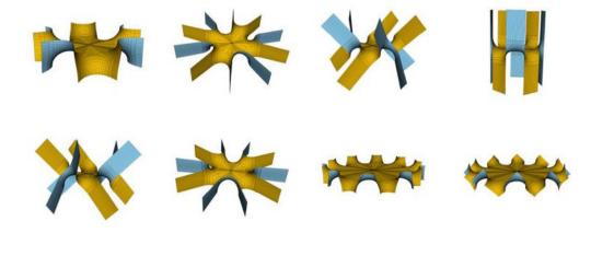
A minimal surface is that which the mean curvature of the surface equals 0. Thefore it gives the surface the ability to reduce material and become structuraly self supporting.
