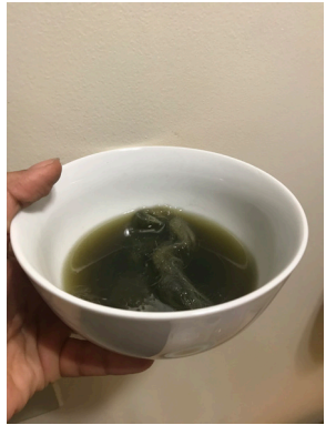
A piece of wool immersed in the Basil dye with Iron as a mordant.
