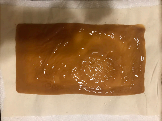
The bioleather kept on a piece of muslin, which is porous, and would help dry the leather faster.
