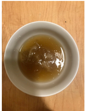
The addition of Alum as a mordant didn't bring much of a colour difference, which is good to get the actual colour of the Basil dye.
