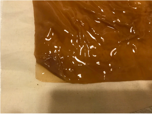
One of the upper layers of the bioleather being folded to show the bottom layer of the bioleather.
