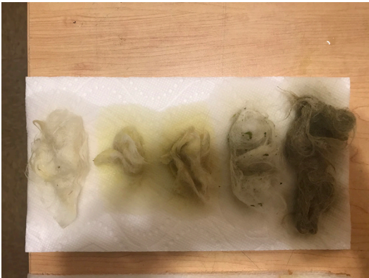
The dyed wool pieces obtained from the Spinach dye; Mordants from left to right: Tartaric acid, Alum, no mordant, soda ash, Iron.
